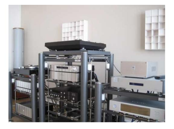
Initially on top of the sturdy Wadia, for critical listening, the LPU 1 was placed on its own level.
