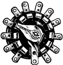
Suitable for many applications such as crystal and band-switching, switching tapped transformer primaries, meter switching, etc. All porcelain construction, ample insulation to handle heavy currents and high voltages. Units with four to eight points are only 2 3/4" in diameter; switches with nine to twelve points are 3 3/4" in diameter. Made in
