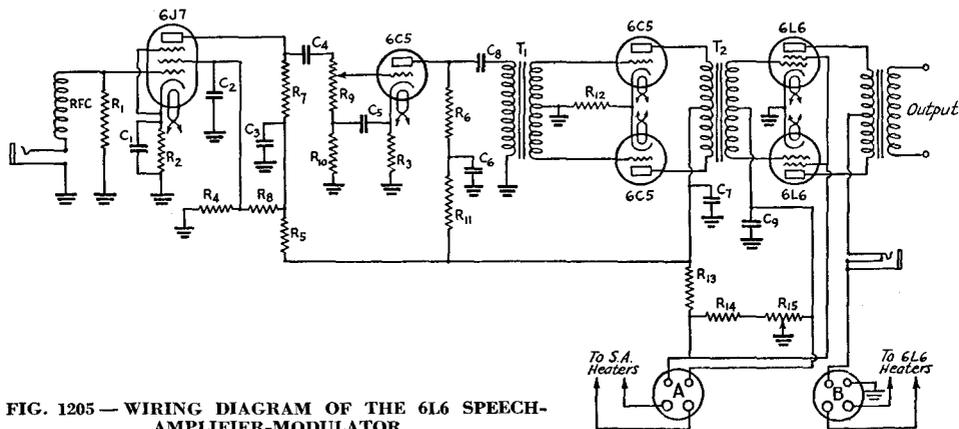
FIG. 1205 — WIRING DIAGRAM OF THE 6L6 SPEECH-AMPLIFIER-MODULATOR
