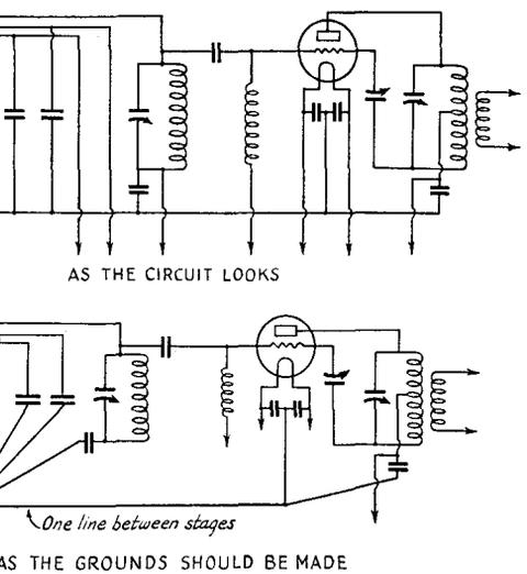
FIG. 907 — WHEN THE TRANSMITTER IS BUILT ON INSULATING MATERIAL, GROUND LEADS FOR EACH STAGE SHOULD BE BROUGHT TO ONE POINT, WITH GROUND CONNECTIONS BETWEEN STAGES MADE AS SHOWN
