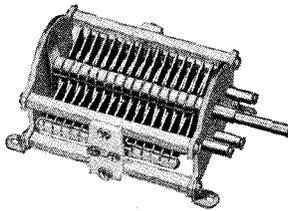
Compact types. Isolantite insulation. Base or panel mounting. Polished aluminum plates. Stainless steel shaft. Size of 150 mmf. with .070" plate spacing only 4 1/2" behind panel. "A" model has .040" plate thickness, all others .025". "A" and "B" models — rounded plates. "C" types — plain plate edges. Self-cleaning wiping contact.
