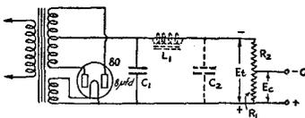
FIG. 1514 — A PRACTICAL CIRCUIT FOR THE "C" SUPPLY
