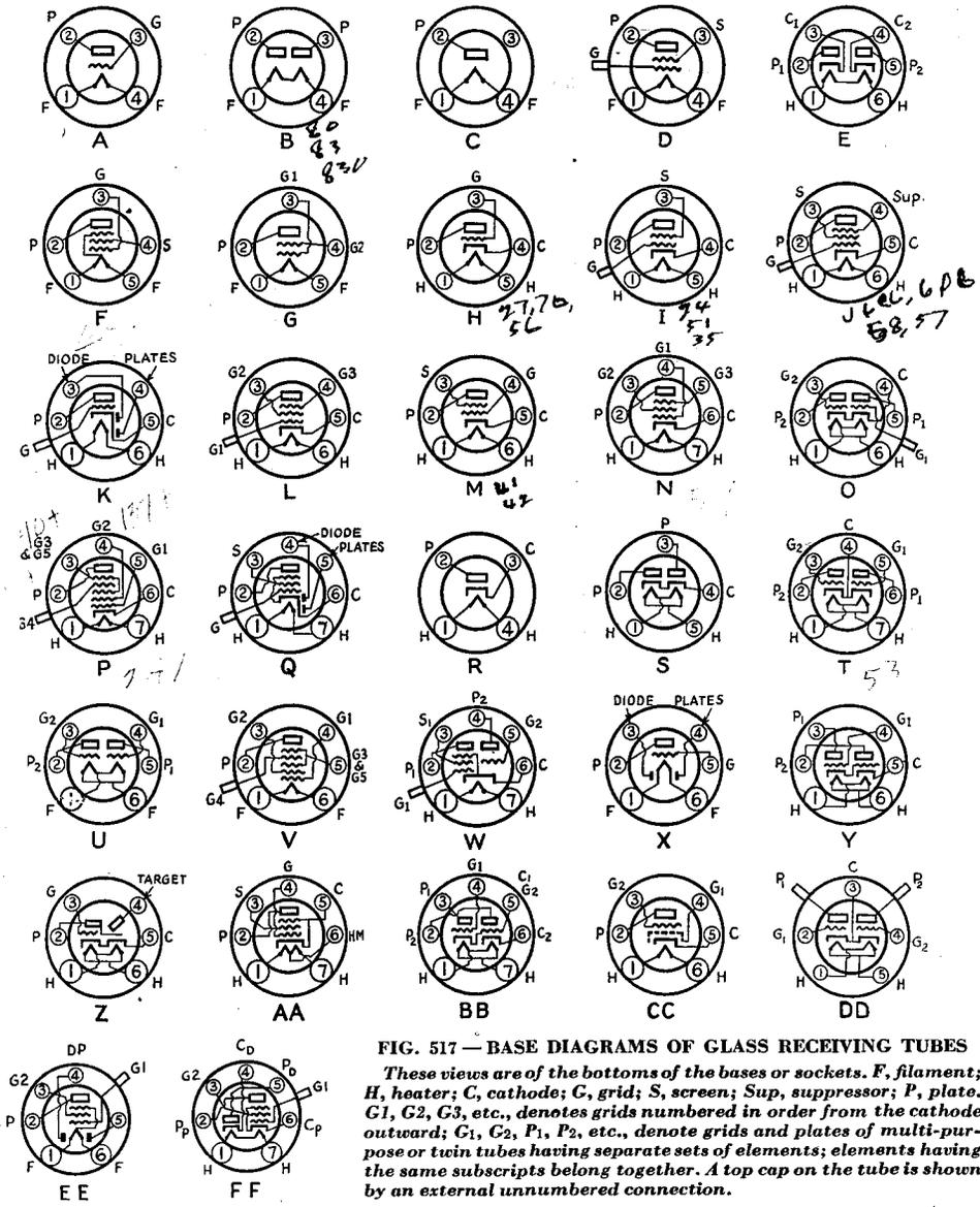
**FIG. 517 — BASE DIAGRAMS OF GLASS RECEIVING TUBES**
