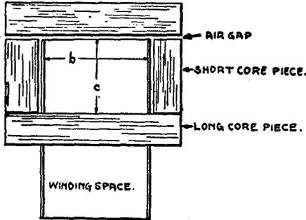
FIG. 1525 — CORE ARRANGEMENT FOR FILTER CHOKE COILS
