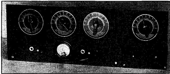
FIG. 911 — PANEL VIEW OF THE 47-46-10 TRANSMITTER WITH ITS ANTENNA-TUNING UNIT
