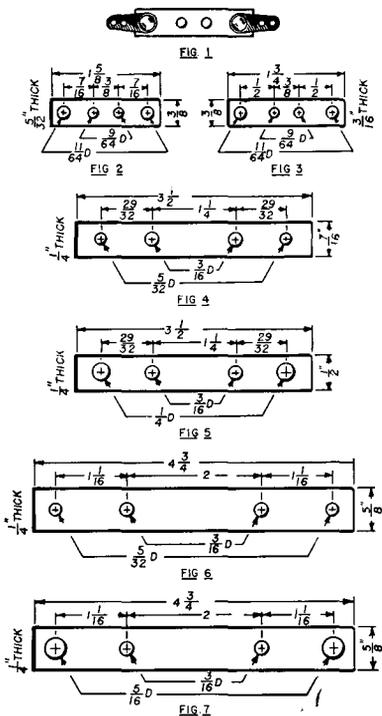
**INSULATORS:** A number of our standard condenser insulators are shown above. In addition to their obvious use as repair parts they may be used for a variety of other purposes such as supports for coils, spreaders, etc. The insulator shown in Fig. 1 is the same as Fig. 3, but has a metal solder lug riveted to each end. It is useful as a 5-meter lead-in spreader, or as a mounting for 5-meter inductances.
