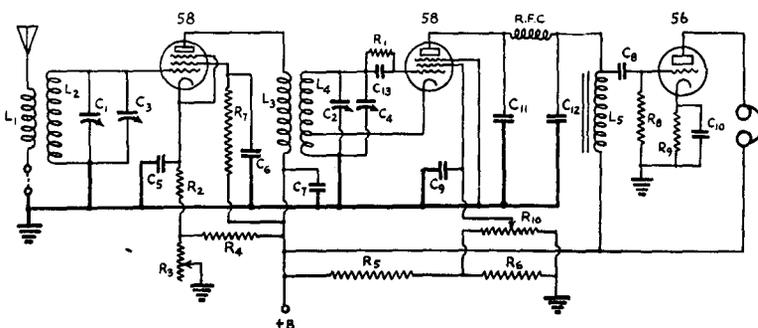
FIG. 713-A — CIRCUIT DIAGRAM OF THE "OLD RELIABLE" RECEIVER
