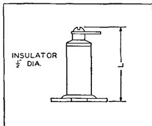
**STAND-OFF INSULATOR.** This well-known little insulator is now offered in two lengths. Long and slender, the larger model is shaped for extreme electrical efficiency. It is an excellent core for H.F. solenoid chokes. (Isolanite)
