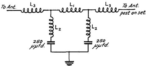
FIG. 1014 — CIRCUIT DIAGRAM OF SHARP CUT-OFF LOW-PASS FILTER
