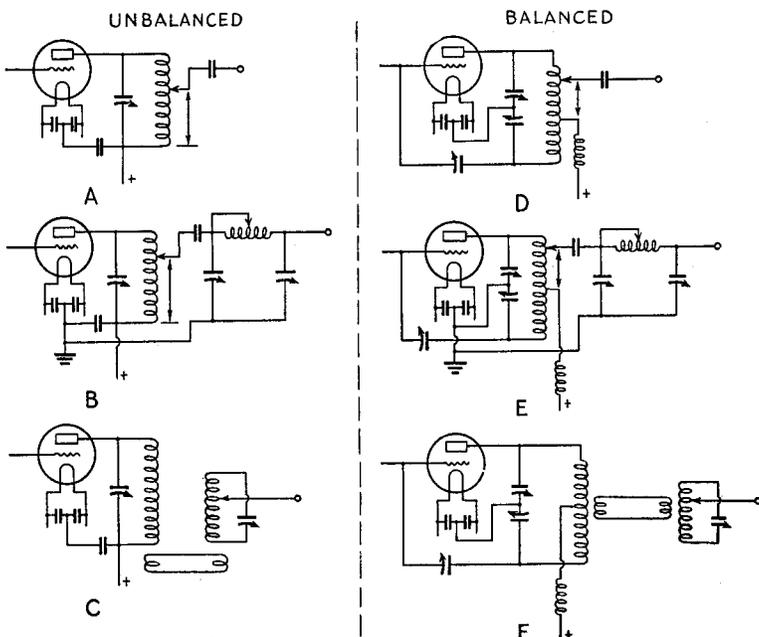
FIG. 1613 — COUPLING THE SINGLE WIRE
