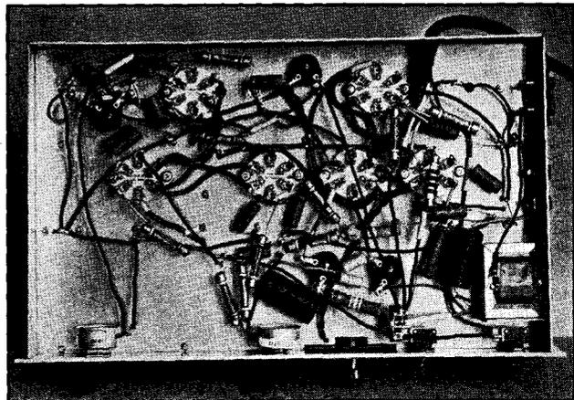
FIG. 721 — A BOTTOM VIEW OF THE SIX-TUBE SUPERHET
