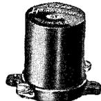
Popular R.F. choke with special impregnated helical winding enclosed in bakelite case,  $1\frac{13}{16}''$  high and  $1\frac{5}{16}''$  in diameter. Ideal for detector plate circuit and R.F. filtering systems in general. Two types—85 mh. with dist. cap. of 3 mmf. and D.C. res. of 250 ohms, and 250 mh. with dist. cap. of 2 mmf. and D.C. res. of 420 ohms. Current carrying cap. of both types 60 ma.
