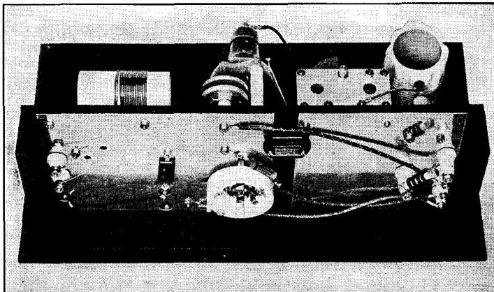
FIG. 939 — A BOTTOM VIEW OF THE SINGLE-TUBE AMPLIFIER
