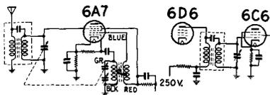
The 6A7 circuit may use any of the 500 series of antenna couplers and the 2000 oscillator coil. The r-f interstage circuit between a 6D6 and 6C6 uses the 1000 series of r-f coils. In this circuit include a 1000-ohm resistance and 0.1 uf. condenser in the plate supply lead to insure stability at high gain.
