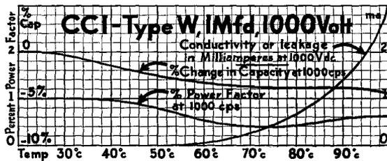
Characteristic curves of the CONTINENTAL Carbon Type W transmitting condensers indicate the excellent performance of these capacitors.
