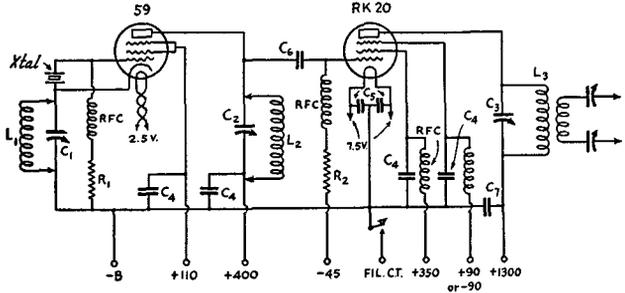
FIG. 925 — CIRCUIT DIAGRAM OF THE TWO-STAGE PENTODE TRANSMITTER
