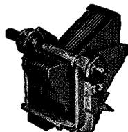
Here is the popular midline condenser which has become a by-word in radio. It has specially shaped brass plates, full floating rotor, removable shaft, perfect bearings and contact, with a rib re-inforced aluminum alloy frame. Isolantite insulation used exclusively. These condensers can be supplied in dual types upon special order. Straight frequency line available on order.
