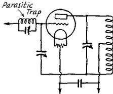
FIG. 829 — ULTRA-HIGH FREQUENCY TRAP TO ELIMINATE PARASITIC OSCILLATIONS
