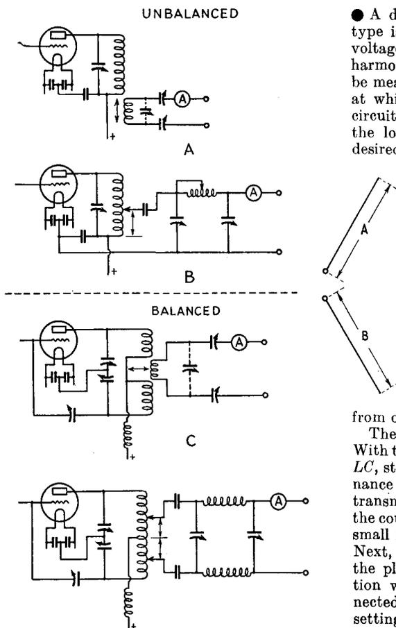
FIG. 1604—DIRECTLY EXCITED ANTENNA—CENTER-FED WITH SUITABLE COUPLING ARRANGEMENTS
