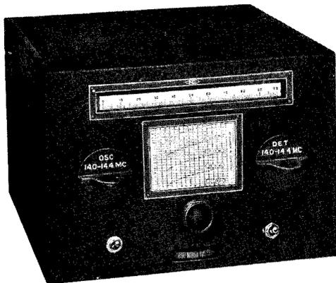
The FB-7 is a seven tube receiver having exceptional sensitivity, selectivity and stability. Ample sensitivity and selectivity are assured through the use of a circuit employing two stages of high-gain air-tuned I.F. amplification. There is no pulling-in or blocking by strong local signals, and frequency drift in both high frequency and beat oscillators has been virtually eliminated. Variation of the volume control has no appreciable effect on the pitch of C.W. signals, even at 14 mc.
