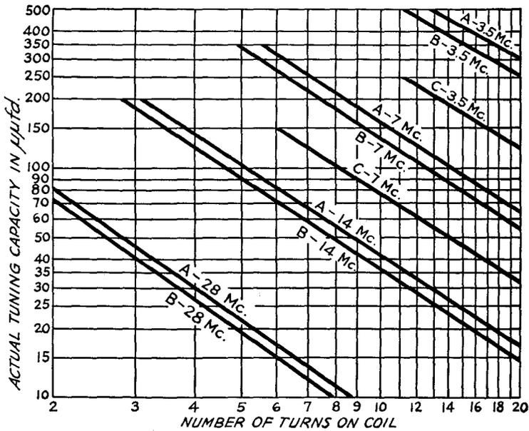
FIG. 832 — WINDING DATA FOR COPPER-TUBING COILS
