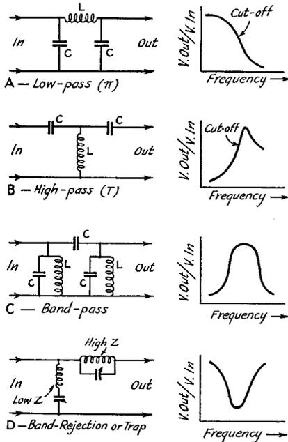
FIG. 410 — TYPES OF FILTERS AND APPROXIMATE CHARACTERISTICS OF EACH
