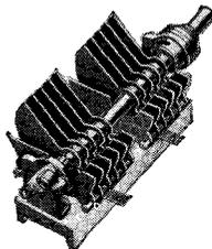
Identical to split-stator condensers except that plates are widely spaced—actual air gap between rotor and stator plates — .0715". No shield between stators. Equipped with new Hammarlund noiseless wiping contact, and split type rear bearing. Condenser ideal for ultra-high frequency transmitters using up to 245's or 210's in push-pull.
