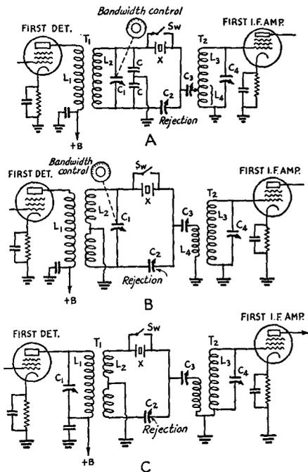
FIG. 621 — THREE TYPES OF CRYSTAL FILTER CIRCUITS
