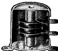
For use in high gain circuits. Universal impregnated wound pies enclosed in an aluminum shield  $1\frac{1}{2}''$  high  $\times$   $1\frac{3}{8}''$  in diameter. Mounting legs on  $1\frac{11}{16}''$  center. Connections to terminal are on one side of the can properly indicated. Inductance—10 mh. D.C. resistance—65 ohms. Current carrying capacity—100 ma.
