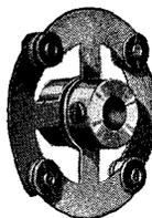
This coupling permits tandem operation of any number of independent units without requiring exact shaft alignment. A great convenience and time saver. The sides of the condenser are insulated from each other, allowing instruments in gang to be operated as independent electrical units. Bakelized canvas with brass bushings for  $\frac{1}{4}''$  shaft. Four rust proofed and hardened steel set screws provide against shafts slipping. Overall diameter  $1\frac{1}{2}''$ .
