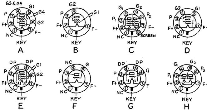
FIG. 518-A — SOCKET-CONNECTION DIAGRAMS FOR OCTAL-BASED 2.0-VOLT TUBES
