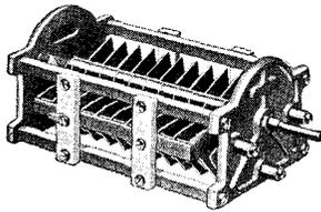
End plates of heavy cast aluminum. Isolantite cross bars. Non-inductive, self cleaning wiping contact. Polished heavy aluminum plates, accurately spaced. Round edged for extremely high voltage work. "A" types — 6500 V — .192" plate spacing; "B" types — 3000 V — .080" spacing; "BX" type — 3500 V — .100" spacing; "X" types — 2000 V — .080" spacing, and "C" types —
