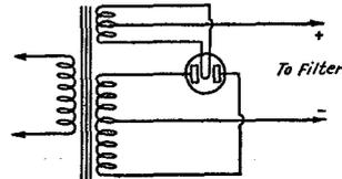
FIG. 1503 — HOW FULL-WAVE TUBE RECTIFIERS ARE CONNECTED
