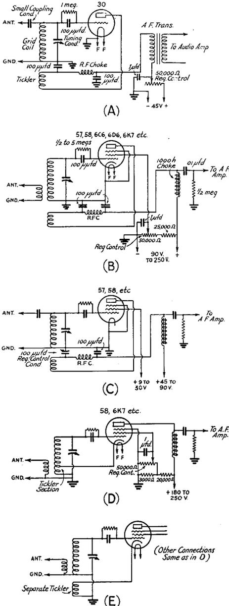
FIG. 604 — TRIODE AND PENTODE (SCREEN-GRID) REGENERATIVE DETECTOR CIRCUITS
