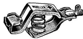
A medium sized clip for connections to storage batteries. Heavy, flanged construction. Lead Plated. Copper shunt protects spring. 25 Amperes.  $2\frac{7}{8}$ " long. Jaw spread 1".
