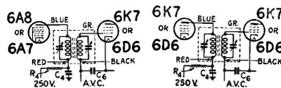
A resistor (1000-1500 ohms) by-passed by a condenser (0.1 uf) appears in the plate circuits. This is recommended because the high gain of Polyron transformers may cause oscillation if stray coupling exists.
