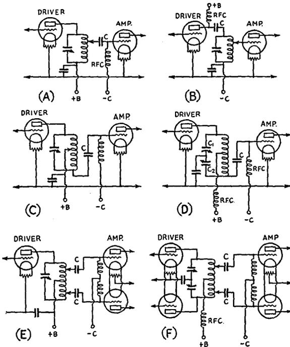
FIG. 814—DIRECT OR CAPACITY-COUPLED DRIVER AND AMPLIFIER STAGES
