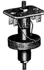
The use of ALADDIN Polyiron adjustable cores in Type K choke coils increases the range of application of these inductors. In experimental work critical values of inductance may be required — a slight movement of the adjustable Polyiron core quickly secures the desired value. Current in excess of 15 ma. is not recommended.
