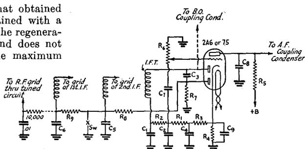
FIG. 626 — THE SECOND DETECTOR-A.G.C.-FIRST AUDIO CIRCUIT
