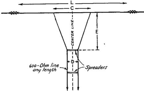
FIG. 1615 — TWO-WIRE MATCHED-IMPEDANCE ANTENNA SYSTEM
