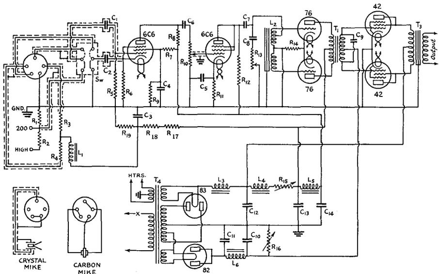
FIG. 1203 — CIRCUIT OF THE GENERAL-PURPOSE 18-WATT AUDIO UNIT
