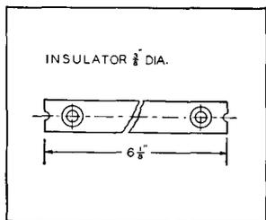
**SPREADER:** The unusual efficiency of these Steatite spreaders will more than justify their slight extra cost. The six inch line spacing when used with No. 12 wire will give feeders having a surge impedance of 600 ohms.
