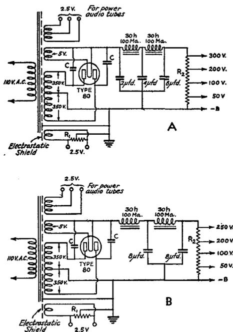
FIG. 1516 — WIRING DIAGRAMS FOR RECEIVER POWER SUPPLIES
