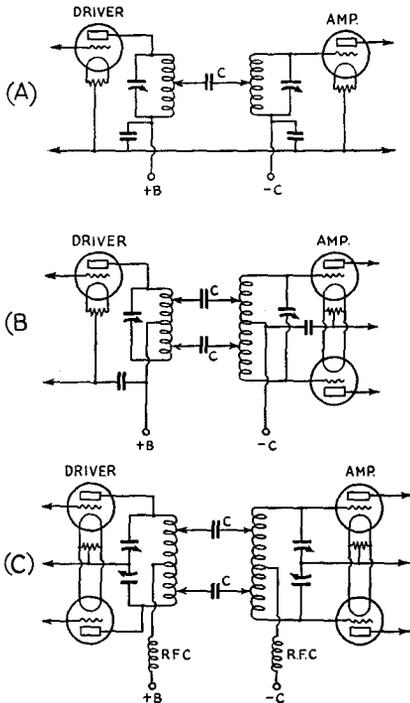
**FIG. 816 — TRANSMISSION-LINE OR "MATCHED IMPEDANCE" COUPLING**
