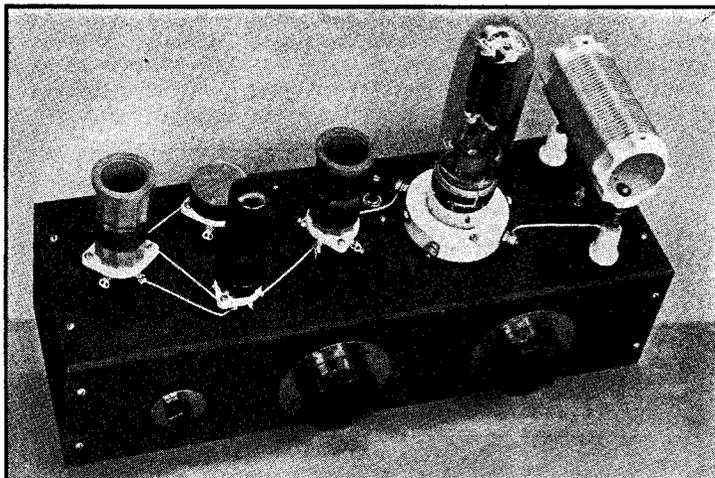
**FIG. 934 — A TWO-STAGE 100-WATT TRANSMITTER FOR THREE BANDS**
