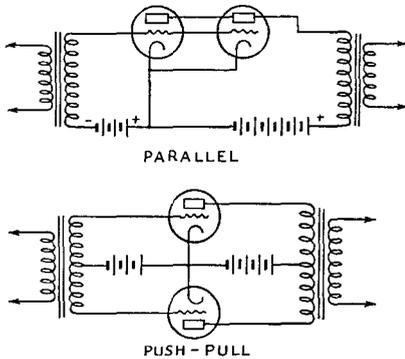
FIG. 506 — PARALLEL AND PUSH-PULL AMPLIFIER CONNECTIONS
