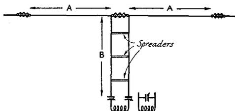
FIG. 1609 — CENTER-FED ANTENNA WITH TUNED FEEDERS
