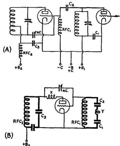
FIG. 826 — HOW LOW-FREQUENCY PARASITIC OSCILLATIONS CAN BE GENERATED
