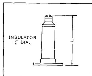
**STAND-OFF INSULATOR.** Metal mounted like the smaller units, these heavy Isolanite stand-offs combine electrical efficiency with strength and convenience. The insulator is  $\frac{3}{4}$ " diameter and is available in two lengths.
