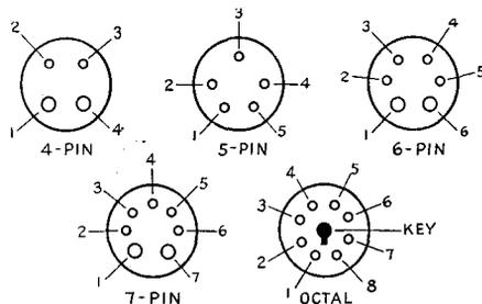
FIG. 516 — TUBE-BASE PIN NUMBERING SYSTEM
