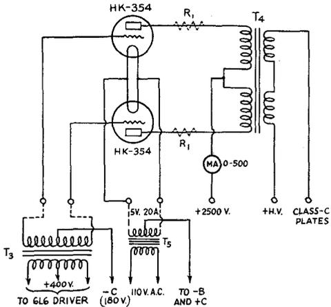
FIG. 1211 — CIRCUIT OF THE 500-WATT CLASS-B MODULATOR
