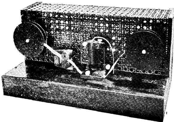
The first and the only automatic code machine using photo-electric cell.
