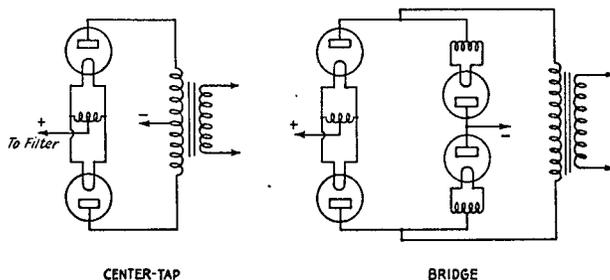
**FIG. 1504 — CENTER-TAP AND BRIDGE RECTIFIER CIRCUITS**
