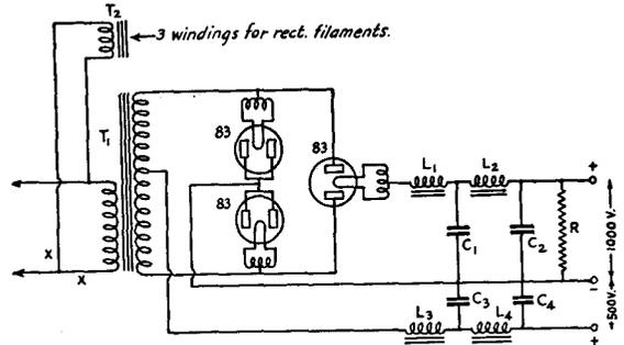
FIG. 1512 — A DUPLEX PLATE SUPPLY CIRCUIT
