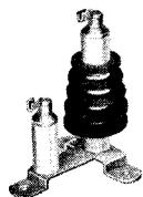
**R-152, R-154, R-154U.** These transmitter chokes have honeycomb coils (0.6 amps. rating) wound on Isolantite cores. The R-152 is designed for the 80 and 160 meter bands; inductance 4 m.h., D.C. resistance 10 ohms. The R-154 and R-154U give maximum impedance on the 20, 40 and 80 meter bands; inductance 1 m.h., D.C. resistance 6 ohms. The R-152 and R-154 are as illustrated. The R-154U does not have the small insulating pillar and the third mounting foot.
