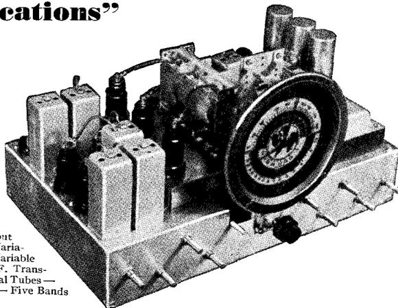
The complete Coil Kit consists of the following: Completely wired tuning unit as described above. Noise Silencer I.F. Transformer. Beat Frequency Oscillator Transformer. Matched Pair of Crystal Filter Transformers. FERROCART (Iron-Core) I.F. Output Transformer. Band Expansion I.F. Transformer. FERROCART (Iron-Core). 6 Shielded R.F. Chokes. Complete set of diagrams and instruction sheets.
