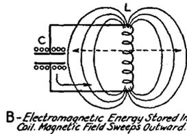
B - *Electromagnetic Energy Stored In Coil. Magnetic Field Sweeps Outward.*
