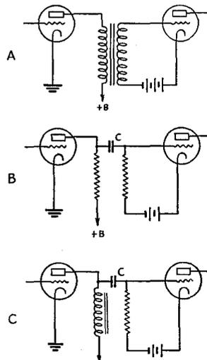
FIG. 507 — METHODS OF COUPLING BETWEEN AMPLIFIER TUBES
