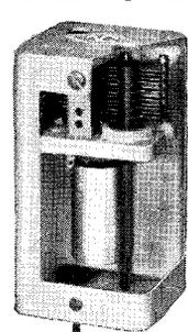
Mounted on the Isolantite base are two 25 mmf. condensers (2000 volts — isolated from each other by an aluminum shield) and an R-39 coil form (1 1/2" x 1" diameter). The assembly is enclosed in an aluminum can, 4" x 2 3/8" x 2". This unit is also available with the Plug-In Base shown on page 9 which makes it ideal for conveniently and rapidly changing transmitting frequencies.
