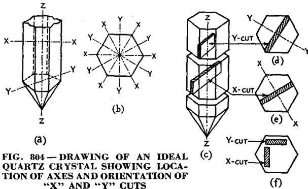
FIG. 804 — DRAWING OF AN IDEAL QUARTZ CRYSTAL SHOWING LOCATION OF AXES AND ORIENTATION OF "X" AND "Y" CUTS
