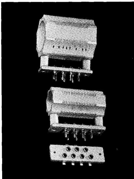
**E**NTHUSIASTICALLY indorsed by thousands of users, these coil forms are standard in low- and medium-power amateur oscillator and amplifier circuits.
