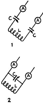
**FIG. 1607 — SERIES AND PARALLEL FEEDER TUNING**
