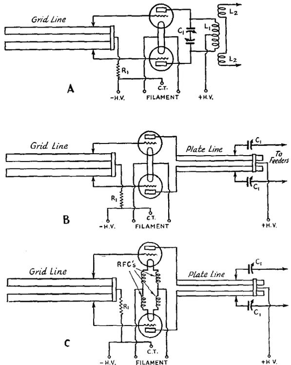
a quarter wave — it would be exactly a quarter wave if it were not for the loading offered by the capacity of the vacuum-tube elements.
