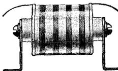
For S.W. and ultra-S.W. receivers and transmitters. Effective over broadcast band too. Recommended as grid choke for multistage transmitters. Isolantite spool. Four sectionalized windings, moisture proofed protected by radio frequency lacquer and cellophane covering. Choke  $\frac{13}{16}'' \times \frac{7}{16}''$ . Flexible leads. Removable brackets.
