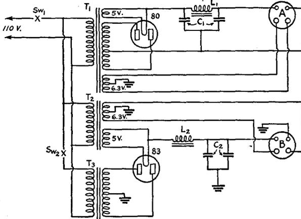
FIG. 1206 — DIAGRAM OF THE 6L6 POWER-SUPPLY UNIT
