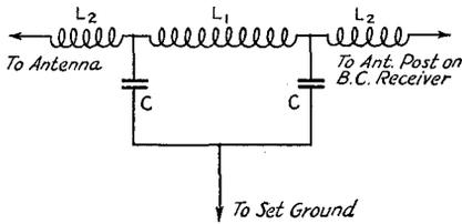
FIG. 1013 — A LOW-PASS FILTER FOR REDUCTION OF INTERFERENCE WITH BROADCAST RECEPTION
