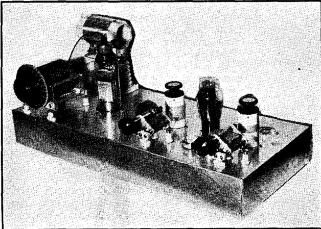
FIG. 924 — A THREE-BAND TWO-STAGE PENTODE TRANSMITTER
