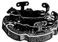
New double Isolantite type with all the outstanding features of the single type. Phosphor bronze flexible plates shaped to provide substantially straight line capacity increase. Constant capacity and power factor maintained under all varying conditions of temperature, humidity, and vibrations. Base  $1\frac{15}{16}''$ . Mounting centers  $1\frac{1}{2}''$ .
