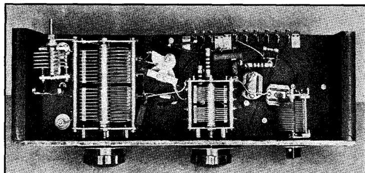
FIG. 936 — A BELOW-BASE VIEW OF THE 100-WATT TRANSMITTER
