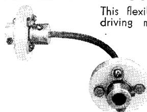
This flexible shaft, providing a driving means between offset shafts or shafts at angles up to 90 degrees, virtually eliminates mis-alignment problems. Available with either plain hubs or with Isolantite insulation. Hubs fit 1/4" shafts.
