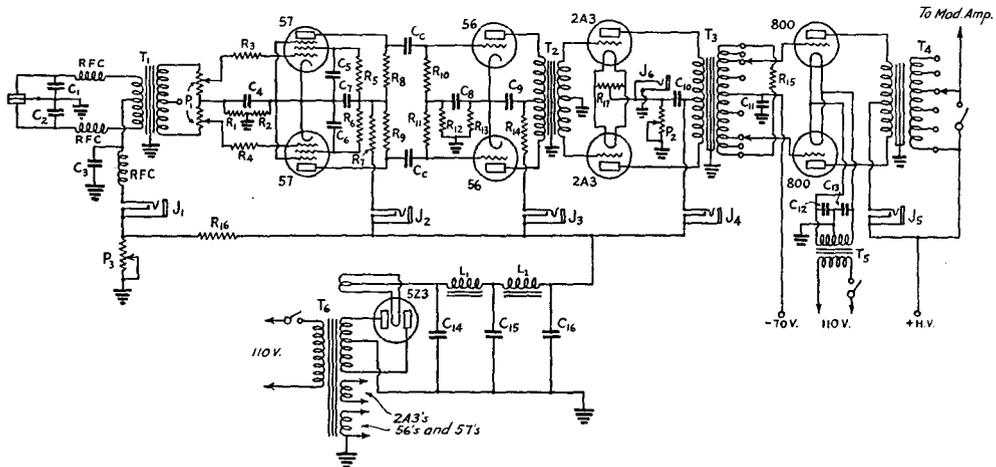
FIG. 1209 — CIRCUIT OF THE 100-WATT AUDIO SECTION
