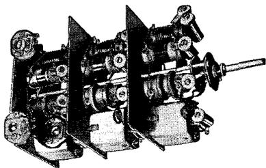
In answer to the constant demand for an "All Wave" coil assembly that will meet the demands of modern requirements, Meissner offers the coil and switch assembly as shown in the illustration.
