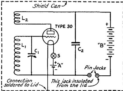
FIG. 1703 — WIRING DIAGRAM OF THE MONITOR
