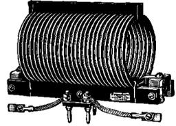
The Plug-in series is so designed that all amateur bands from 10 to 160 meters may be covered with one variable condenser with a maximum capacity of 100 µf. They are equipped with two No. 77 and three No. 75 plugs (two of which attach to flexible leads and LC4 Clips for an integral coupling winding) and mount on two 4576J and three 40J Johnson Insulators (see page 506).
