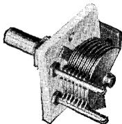
For tuning or trimming on high frequencies. Cadmium plated soldered brass plates. B-100 Isolantite. Base mounting, single hole panel mount, or panel mounting with bushings. 140 mmf. size 1 9/16" high, 1 13/16" behind panel.
