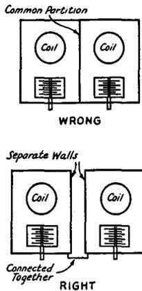
FIG. 606 — SHIELDING COMPLETE ABOUT EACH GROUP OF APPARATUS
