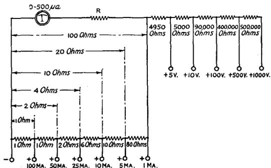
FIG. 1711 — A MULTI-RANGE VOLTMETER-MILLIAMMETER USING A 0-500 MICROAMMETER
