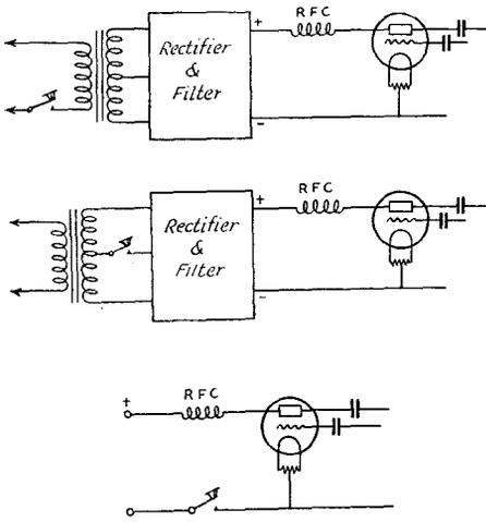
FIG. 1001 — PLATE-KEYING METHODS
