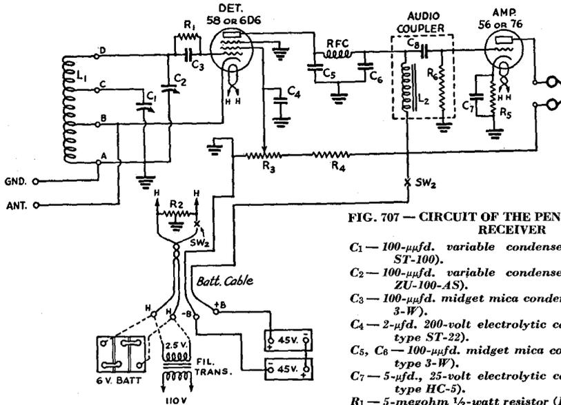
**FIG. 707 — CIRCUIT OF THE PENTODE DETECTOR RECEIVER**
