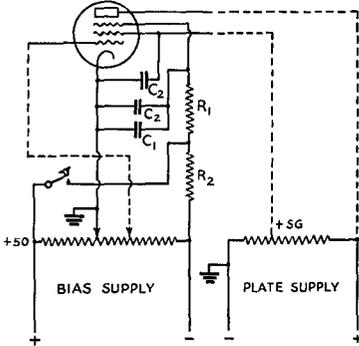
**FIG. 1004 — SUPPRESSOR KEYING OF A PENTODE TRANSMITTING TUBE**
