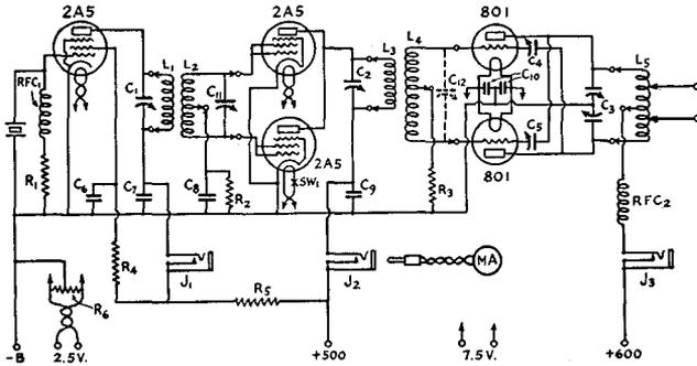
The panel controls, from left to right, are the oscillator tuning condenser, on-off switch, *Sw*<sub>1</sub> second-stage tuning condenser, plate current jacks, and finally the amplifier tuning condenser.
